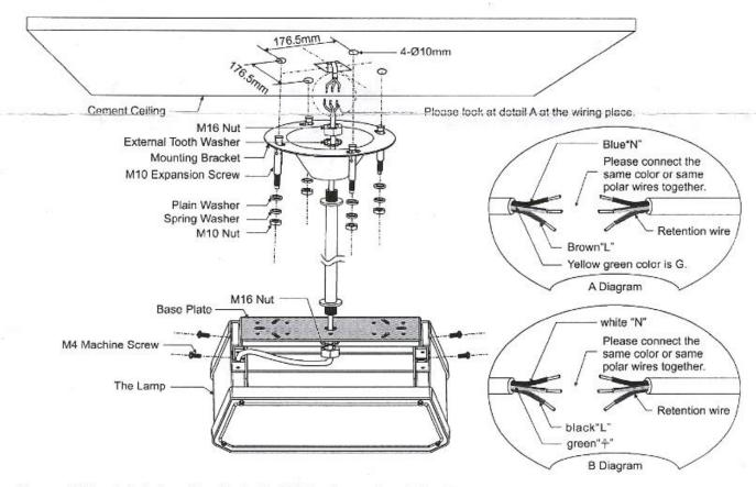
Step one: Drill four holes in the ceiling with electrical drill. Spacing as shown in the picture.
